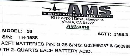
1 REPLACE BOTH ACFT BATTERIES P/N: G-25 S/N'S: G02865087 & G02865089 AND SERVICE WITH 2- QUARTS EACH BATTERY ACID.
